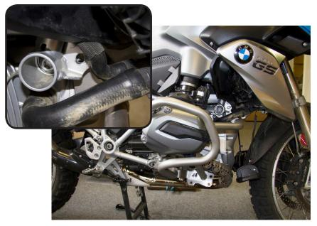
Remove the (2) OEM M10 bolts from frame spar (refer to step 3 for example image). Hang right side crash bars and begin to thread the 2nd M12 nut to hold bars hanging in place. NOTE: front upper mount should be positioned inside the frame unlike the left side which sits outside.
