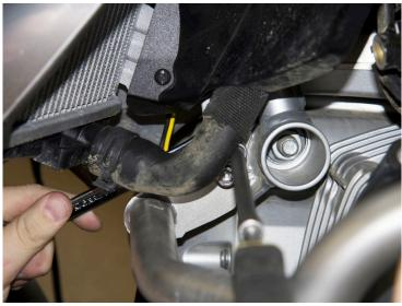
Install the (2) M8 bolts, (4)washer, and (2)lock nuts to the top front mount using an M6 driver and 13mm wrench. Start with the top bolt and tighten most of the way before inserting the bottom bolt to make installation easier. Do not tighten both bolts completely.
