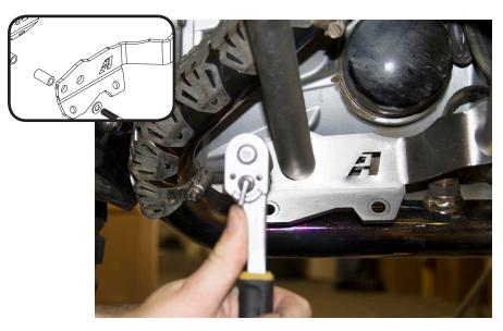
(6) Install the M8 x 50mm bolt with washer, and spacer into the front mount position of the lower bracket. Use anti-seize. Do not torque all the way.
