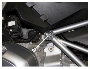
With bike on center stand, remove OEM engine bolt using 18mm socket and T55 driver. Use a 1/4" extension to push the bolt out far enough that you can grab it and remove by hand.
