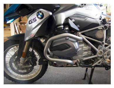
Hang left side crash bars and insert engine bolt from the left side. Do not re-use spacers that come out with OEM bolt.
