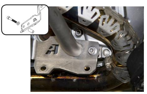
Install the M8 x 50 mm bolt with washer, and spacer into the front mount position of the lower bracket. Use anti-seize. Do not torque all the way.
