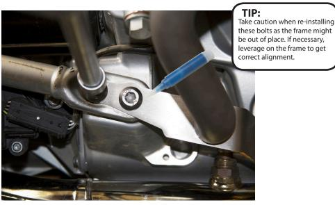
Reinstall the (2) OEM M10 bolts using a T50 driver and clean bolt threads, chase threads in engine, apply thread locker, reinstall and do not tighten all the way. Go back to the front and upper M8 bolts in step 9 and 10 and torque to 10 nm or torque. Return to the (2) OEM M10 bolts and torque to 55 nm or torque.
