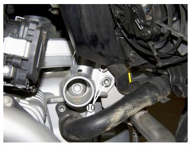
Install the (2) M8 bolts, (4)washer, and (2)lock nuts to the top front mount using an M6 driver and 13mm wrench. Start with the top bolt first and do not tighten all the way. Next start the bottom bolt, washer, and nut combo but do not tighten all the way.
