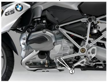
Using a T50 driver remove the (2) OEM M10 lower engine mount bolts on the left side.
