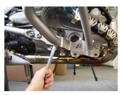
Using a 13mm wrench, tighten all (4) M8 hex bolts holding bars to brackets on each side.
