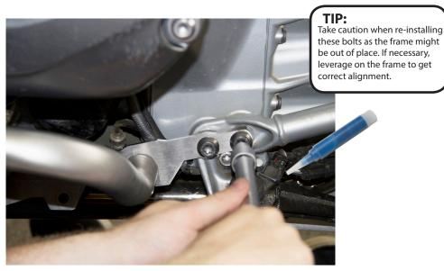
Reinstall the (2) OEM M10 bolts using a T50 driver and clean bolt threads, chase threads in engine, apply thread locker, reinstall and do not tighten all the way. Go back to front and upper M8 bolts in step 5 and 6 and torque to 10 nm or torque. Return to the (2) OEM M10 bolts and torque to 55 nm or torque.
