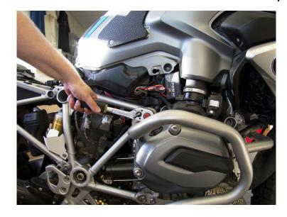
Using two 18 mm sockets, tighten the M12 engine bolt and then torque to 85 nm. Thread locker is not needed on this step because the nut is a locking type nut.
