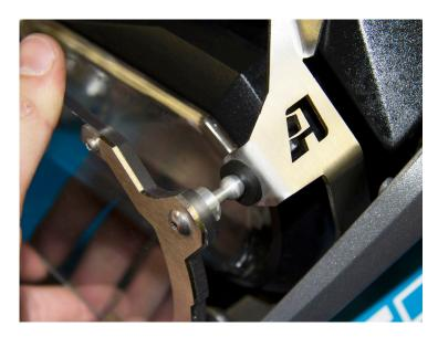
Tighten both OEM T25 fasteners all the way. Then tighten the cap head bolts from underneath with an M5 driver.
