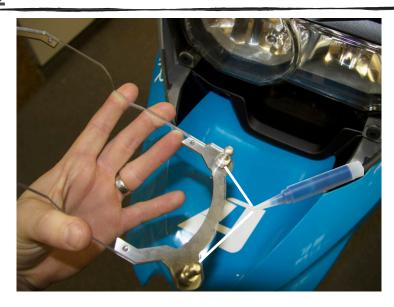
Current headlight guards have ball studs pre-installed. If you have an older version, install ball studs + screws to headlight guard. Apply SMALL drop of loctite into each ball stud. Tighten with bare hands. Hold the ball stud stationary with a 10mm wrench and turn the torx screw 1/4 turn more. Careful, overtightening will crack the lexan.
