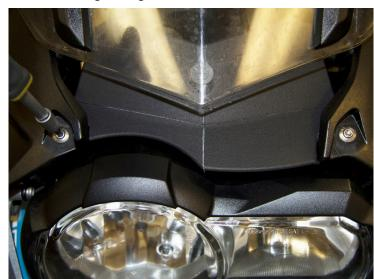
Adjust windscreen to its highest position. Remove the (2) OEM T25 fasteners and set aside. Be careful not to lose the small clear protective plastic behind the screw, you will need this later.
