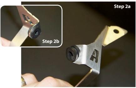
Install the (4) rubber grommets on the right and left side brackets. Sometimes it is easier to get grommets in place if you use some water as lubrication. You can also gently press into place with a flat head screwdriver.
