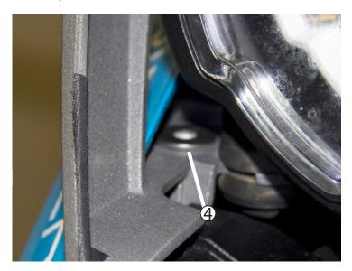
Drop in (2) hat spacers, one on each side into the hexagonal hole in the cast frame. The hole the spacers go in is directly behind the beak fairing. If you are working on a GS Adventure, you will have to flex the palstic out slightly to gain access to this area.
