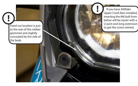
From underneath the beak, insert the cap head bolt with metal washer from the bottom up. The bracket contains a fixed nut that you will thread into. Add a small drop of thread locker to the bolt before starting.
