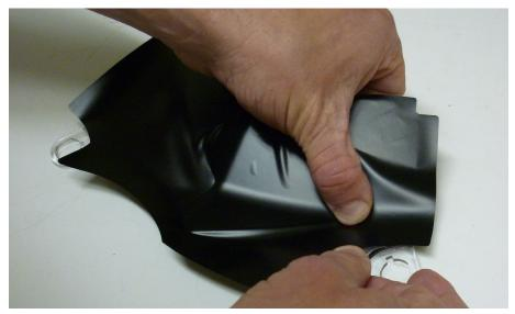
Ontinue to work from the center outward with your thumb or fingers, pressing out bubbles to the edge while lifting with your other hand. It may be lifted and repositioned as necessary to get it to lay smoothly. Large bubbles can be carefully pricked with a sharp exacto knife and pressed flat.
