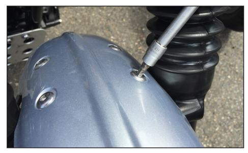
(3) Use a 5 mm Allen tool to remove the (4qty) OEM fender mount bolts shown.
