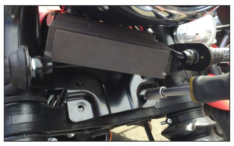
② Use the same 8mm socket tool to remove the two fasteners that hold the turn signal light mount bracket on to the triple clamp. You will need to hold the voltage regulator out of the way while you do this.
