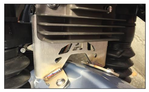
B Double check that all of your fasteners are tight and you are ready to ride. After the first ride go back and doublecheck that all fasteners remain tight and no loosening has occurred.
