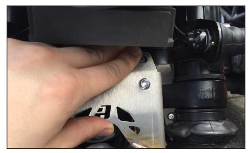
(6) Use the (2qty) M6x20 flathead fasteners provided and mount the upper fender mount bracket as shown using the included (2qty) 8mm spacers to fill the space behind the bracket. (*photo above shows prototype hardware*)
