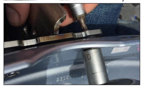
(5) One fastener at a time, slide one of the (4qty) 18mm oversized washers over the shaft of the M6x20mm button head on the underside of the fender, then using a 4 mm allen tool and a 10 mm socket put one of the (4qty) nylock nuts on the shaft and tighten until one thread is past the nylon. Do this for all (4).
