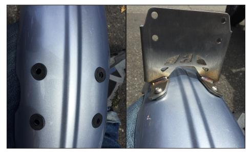
Remove the fender and insert the (4qty) aluminum spacers into the fastener wells as shown *(plastic prototype spacers shown above)*. Now place the high fender mount bracket on top of the aluminum spacers so that the holes align. Insert the (4qty) M6x20 button head fasteners and washers as shown.
