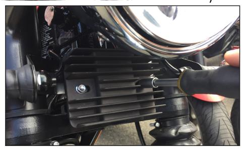
Use an M8 socket driver to remove the (2qty) OEM fasteners that hold the voltage regulator in place. You will be reusing these two fasteners.
