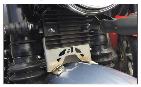
Place the voltage regulator guard back in its place now on top of the fender bracket mount, then using an 8mm socket reinsert and tighten the (2qty) OEM fasteners.
